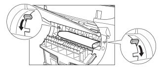
4 Hold both sides of the jammed paper and carefully move it inward, then gently pull it out.
